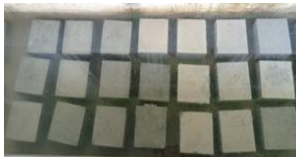
Gambar 4. Proses Perendaman Beton (Curing)
