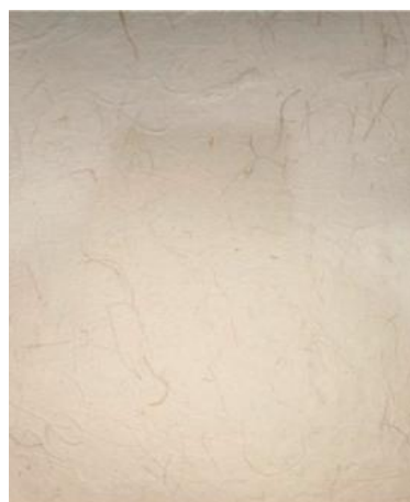
Figure 2. Paper made from corn husk fiber
