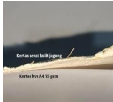
Figure 3. Thickness comparison between corn husk fiber paper and 75 GSM HVS paper
